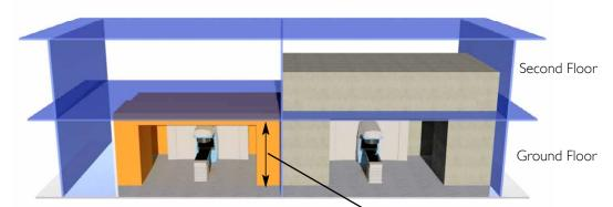
Note: Space saving comparisons shown on left assume unoccupied and unlimited vertical space above the rooms. In projects with occupied conditions above the vaults, actual space savings achievable with VeriShield™ will be significantly higher compared to concrete, as concrete bunkers will extend vertically into the floorspace above - taking up valuable service space.
